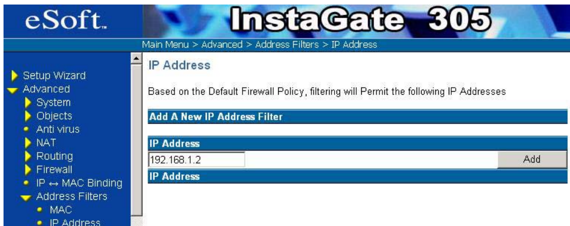
Figure 89: New IP Address Filter
